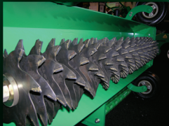
A bottom view of the GBS1200 shows its standard 39 blade setup.
