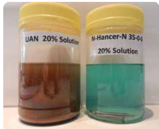
Figure 1. Mild steel nails immersed in 20% strength solutions of UAN and N-Hancer-N for 48 hours
