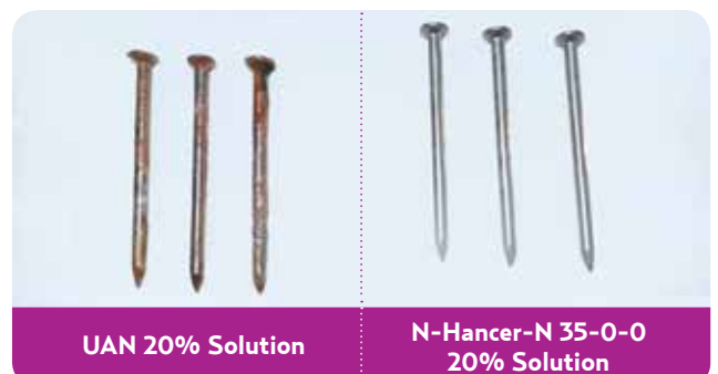
Figure 2. Mild steel nails removed from nitrogen solutions after 48 hours
