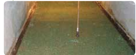
Post-test endurance results concluded that unvegetated GreenArmor 7020 exhibited a critical shear stress of 5.8 lb/ft² (276 N/m²).
